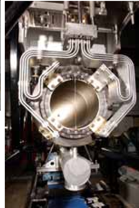
NuMI downstream absorber. Note elaborate cooling. “Cost more than NuTeV beamline...” – R. Bernstein
