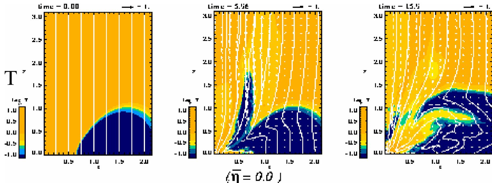
Result of ideal MHD simulation of jet formation by Kuwabara et al. 2000. Jet ejection takes place intermittently due to the growth of MRI in the disk
