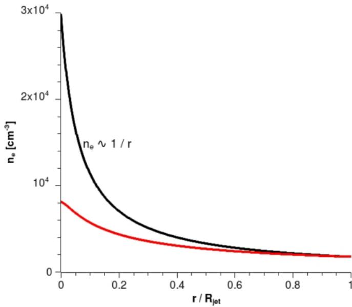
Axisymmetric jet ,  $T_e = 10000 \text{ K}$ ,  $n_e \sim 1/r$
